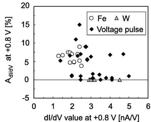
FIG. 2. The asymmetry in  $dI/dV$  curves ( $A_{dI/dV}$ ) at +0.8 V obtained on Mn films thicker than three layers are shown as a function of the  $dI/dV$  value at +0.8 V. All data shown are obtained from  $dI/dV$  curves obtained at a setpoint of  $V_S = -0.5$  V,  $I = 0.5$  nA. Circles, triangles, and diamonds were obtained by different Fe-coated W, different clean W, and different voltage-pulsed tips, respectively.
