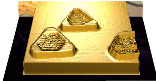
Fig. 3 STM topographic image of Fe nano magnets with a size of about 10-20 nm and a thickness of two atomic layers, which were grown on Cu(111) substrate in UHV.
