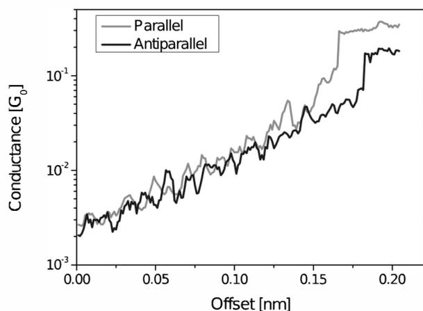
Fig. 4. Two typical single conductance distance curves measured at two contrariwise magnetized islands with a constant tunneling voltage of 10 mV. Below a certain tip-surface separation the curves show a jump of the conductance to higher values. This can be identified by a jump of the molecules into contact. After the jump there are two contributions to the transport.
