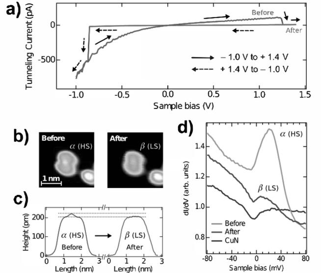
Fig. 7. a)  $I(V)$ -curves of isolated Fe-phen molecules recorded on the center of the molecule. b) STM images c) and corresponding height profiles acquired before and after the switching event. d)  $dI/dV$  spectra recorded on the center of the molecule before and after a switching event.
