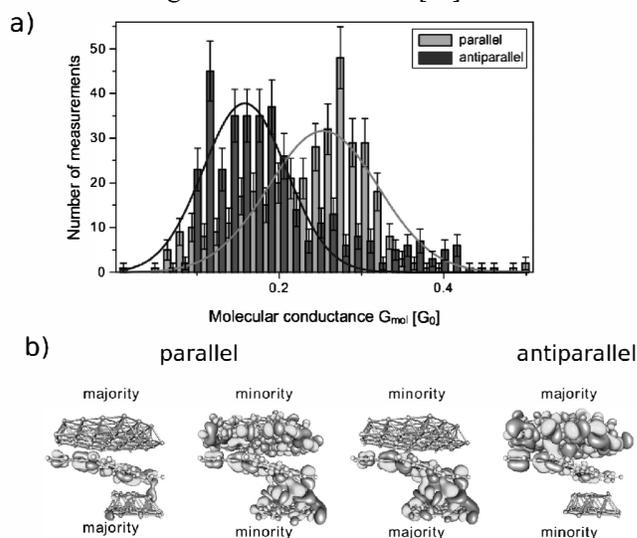
Fig. 5. a) Histogram of the molecular conductances (381 times parallel and 366 times antiparallel). A Gaussian fit is used to determine the conductance and calculate the GMR ratio. b) Calculated electron wave functions for parallel and antiparallel oriented magnetizations for the two spin channels.
