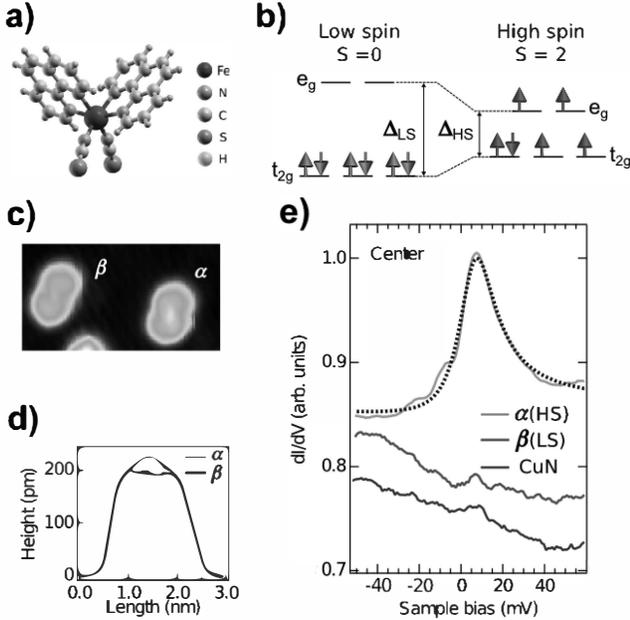
Fig. 6. a) Three dimensional model of an Fe-phen molecule. b) Simplified electronic configuration of the Fe(II)-3d states in the ligand field. c) STM image of isolated Fe-phen molecules on the CuN/Cu(100) surface and d) line scans across the long axis of the molecules. e)  $dI/dV$  spectra taken on the center of the Fe-phen molecules.
